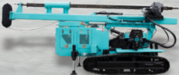
BORED PILE DRILLS EVOMAQ®
