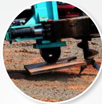
In order to provide greater stability and safety when executing the pile, the turret foot has large dimensions, ensuring higher machine stability and precision when the auger is removed.
