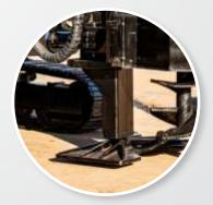
In order to provide greater stability and safety when executing the pile, the turret foot has large dimensions, ensuring higher machine stability and precision when the auger is removed.
