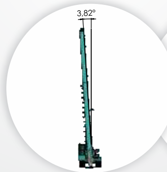
TOWER SIDE SLOPE
